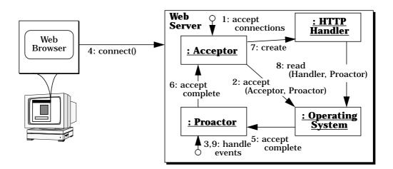
Once the connection is established and the HTTP handler created, the following scenario is used by a proactive Web server to service an HTTP GET request:
